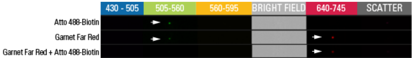
Figure 4. High-resolution detection of EVs using ExoFlow-ONE and conjugated dyes. Streptavidin-coated HEK293T EVs were captured and stained with either biotinylated Atto 488 dye, ExoFlow ONE Garnet Far Red dye, or combination of both dyes. Labeled EVs show correct signals at respective channels optimal for each dye, while bright field and scatter channels show no perceptible signal, indicating the observed event(s) are under the diffraction limit of detection. Data collected using an Amnis® ImageStream X Mark II Flow Cytometer.
